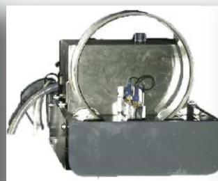
Example of device of measurement of depth of nitriding of bearing
